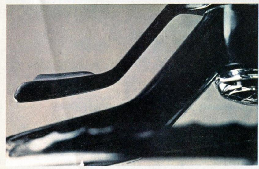
The button on the turn signal lever controls the high and low headlight beams. To dip your lights for an approaching car, just squeeze. No more fishing around on the floor with your foot to find a button.
