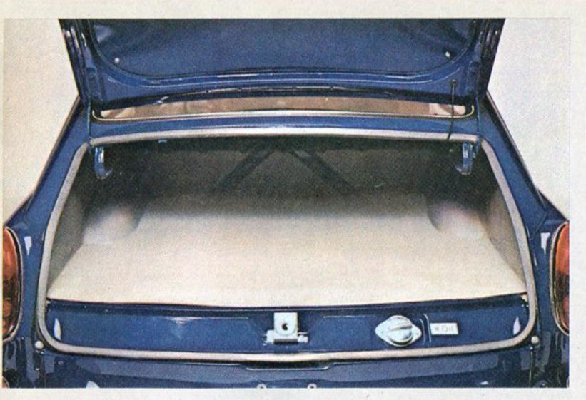
The engine is under the floor of the 10.5-cu.-ft. rear luggage compartment. To check the oil without unpacking the trunk, unscrew the oil cap. (It sits underneath the back door.) A dip stick's attached.
