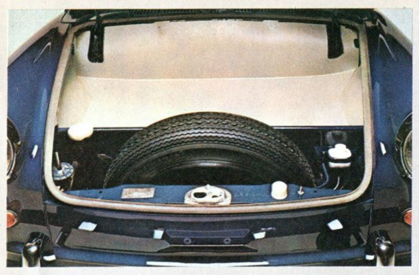
The spare tire sits in front of the forward luggage compartment. You don't have to unload to change a flat. Also up front: easy see-through plastic containers for the brake fluid and windshield-washer water.
