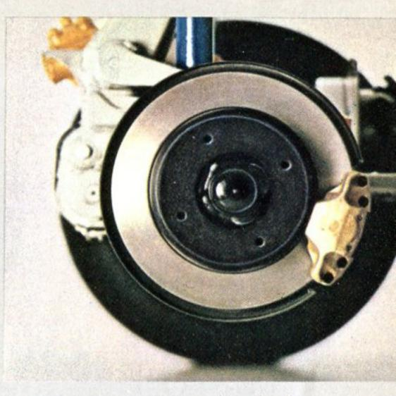
You get even stops, less brake fade with front wheel self-adjusting disc brakes. They're standard equipment.
