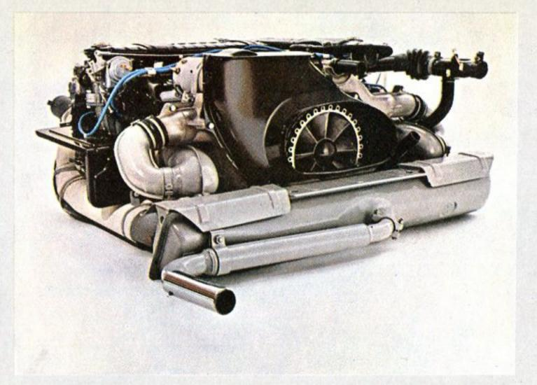
The 4-cylinder engine is cast of light aluminum and magnesium alloys to eliminate dead weight. Pistons travel a short distance at slow speeds to cut down engine friction, lengthen engine life.
