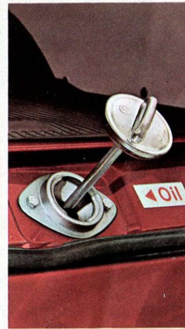
The oil cap (dip-stick attached) is under the back door, outside the engine compartment.
