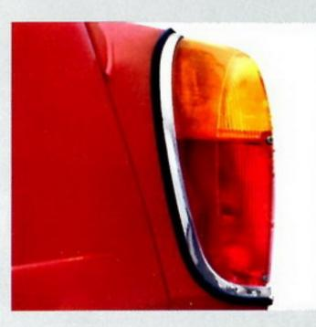
Three divided sections for the turn indicators, tail and brake lights. (Fastened with a rubber strip and chrome ring.)
