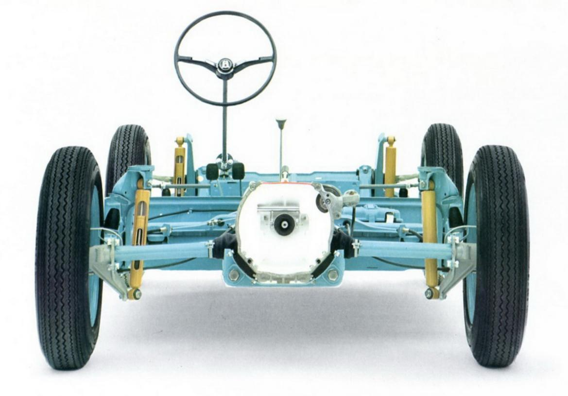
The same principles of suspension apply to the rear wheels: both are independently suspended by divided torsion bars.
