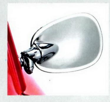
What's so special about this exterior mirror? It's double jointed. It can't snap off when bumped—it just gives way.
