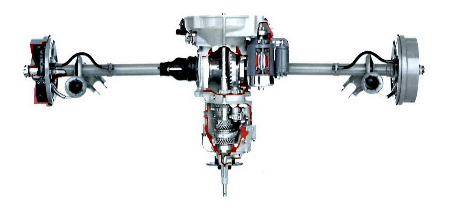
Engine, gearbox and rear axle form a compact unit on the Volkswagen 1500 Sedan and Volkswagen 1500 Station Wagon models (as with every Volkswagen model). That's why the VW doesn't need a drive shaft. Result: the engine's power is transmitted directly to the drive wheels, without loss of power.
