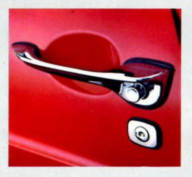
The outside door handles are styled to the car. They are practical, easy to operate—and made of highly rust resistant chrome plated steel.
