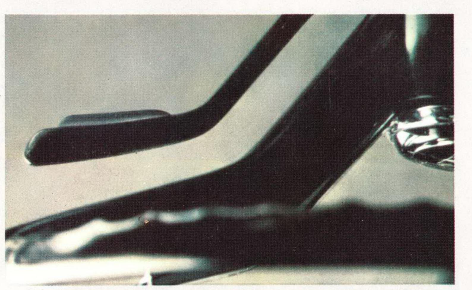
The button on the turn signal lever controls the high and low headlight beams. To dip your lights, just squeeze. No more tromping around with your foot to find a button.
