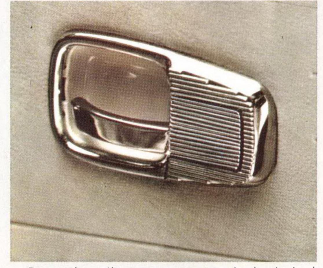
Door handles are recessed. And dashboard knobs and window-crank knobs are flattened out and made of soft rubber.
