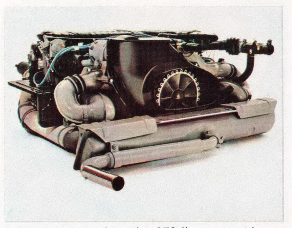
No dead weight in this 270-lb. engine: it's cast of aluminum and magnesium alloys. That's one reason you should get about 27 miles to a gallon.
