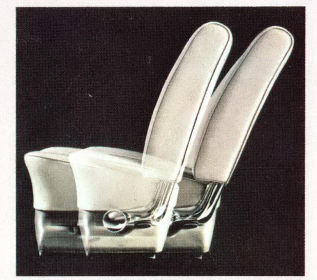
Bucket seats adjust in 7 positions front to rear. Seat backs recline at 7 angles. 49 combinations in all.
