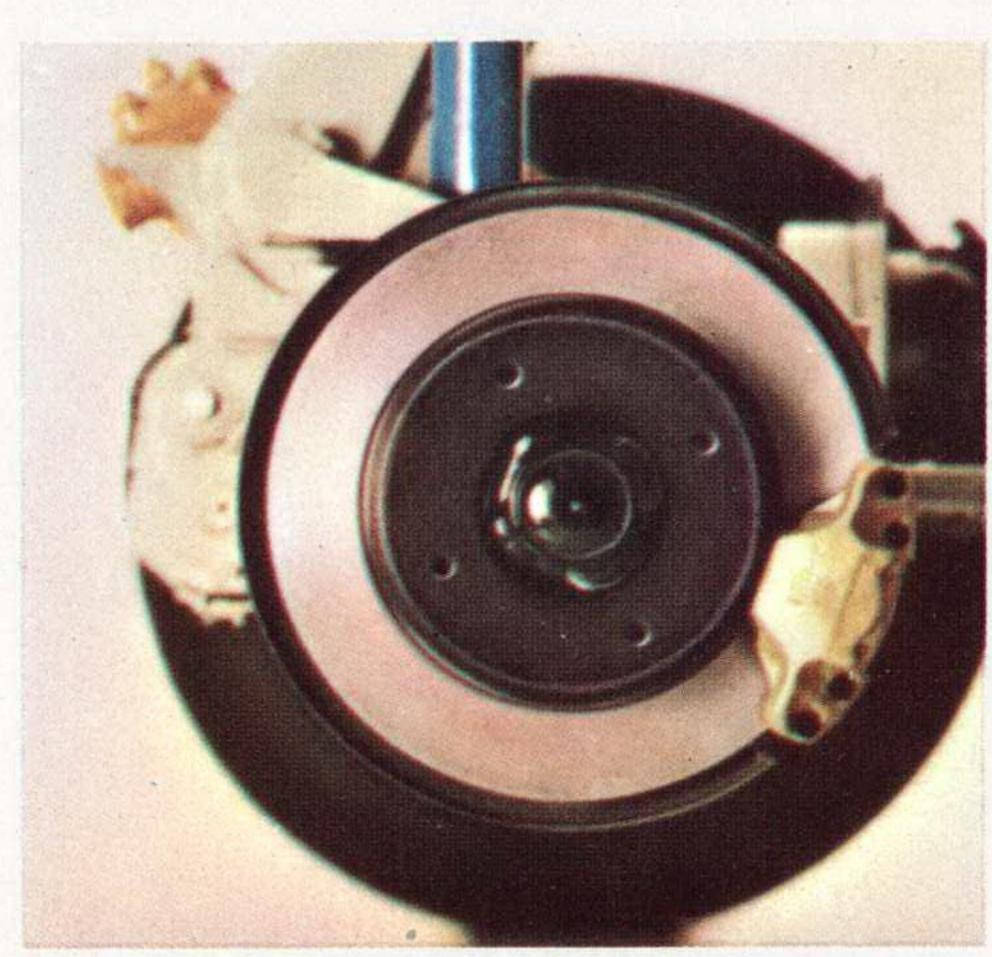
Front wheel self-adjusting disc brakes are half of the dual brake system. They're standard equipment.
